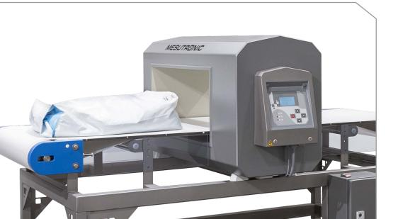
They work as stand-alone machines in the logistics area, usually in combination with **TRANSTRON conveying systems**. They are fed manually; complaints about contaminated bags of the expensive raw materials can be made directly to the supplier without unpacking. Optionally the bags can also either be ejected automatically onto a discharge belt or colour-marked to prevent re-entry into the production process.
